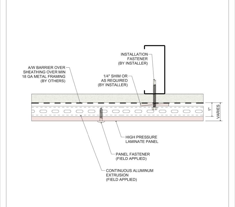
SYSTEM 2000 DETAIL: VERTICAL MID PANEL DETAIL 4
