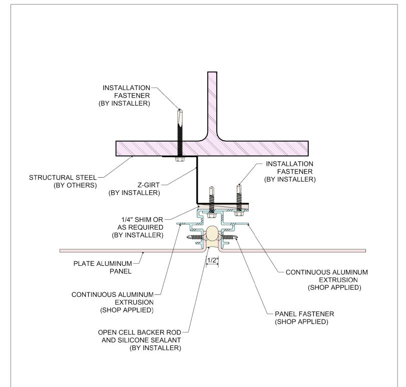
DETAIL: SYSTEM 3150 WET SEAL SYSTEM 12A RECTANGULAR COLUMN DETAIL
