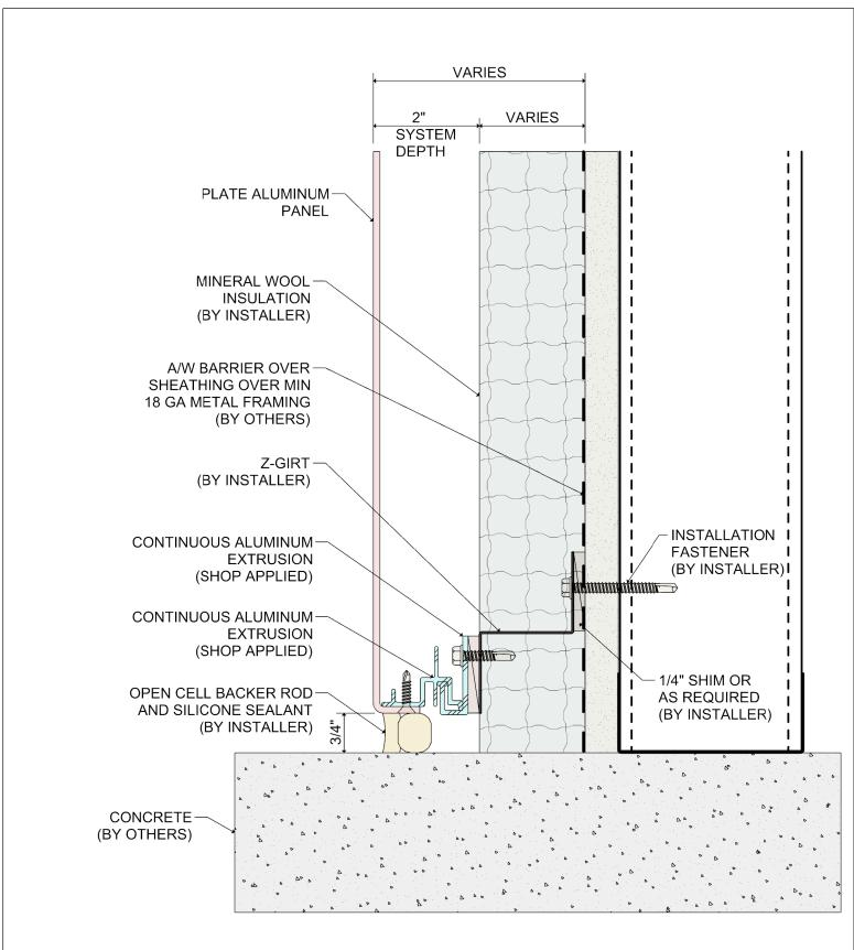
SYSTEM 3150 BASE DETAIL WET SEAL SYSTEM
