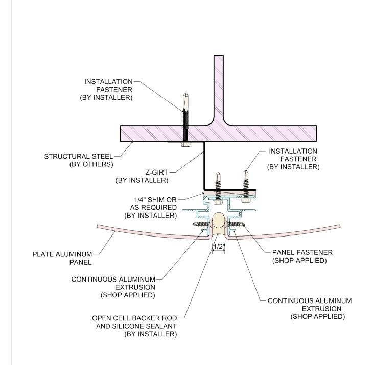
WET SEAL SYSTEM **SYSTEM 3150** DETAIL: **CURVED COLUMN DETAIL**
